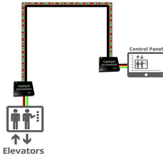
**Figure 3 – Redundant DC-CAN network in elevator application example**
