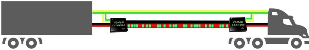
**Figure 2 – Redundant DC-CAN network in Truck – Trailer application example**
