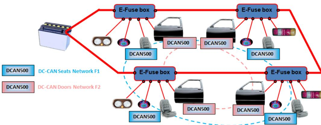
Figure 1 – Redundant DC-CAN network in Vehicle platform application example
