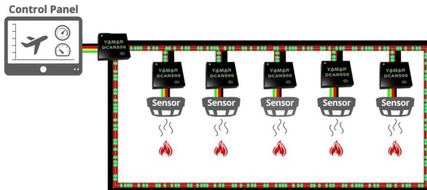
**Figure 4 – Redundant DC-CAN network in sensors application example**
